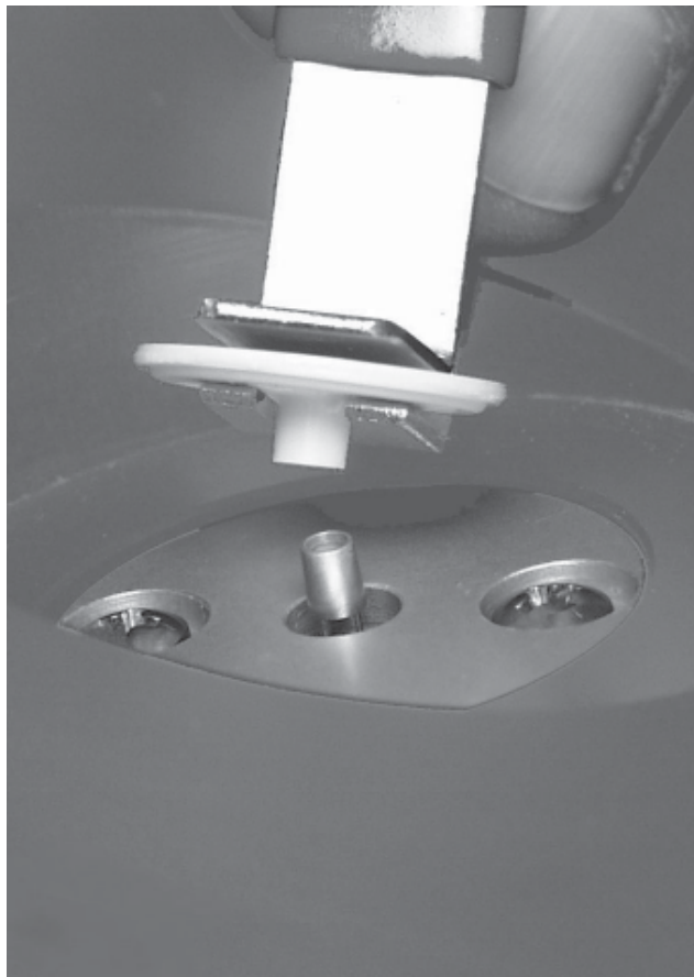
Figure 5-8. Placing the filter on the tapered element.
