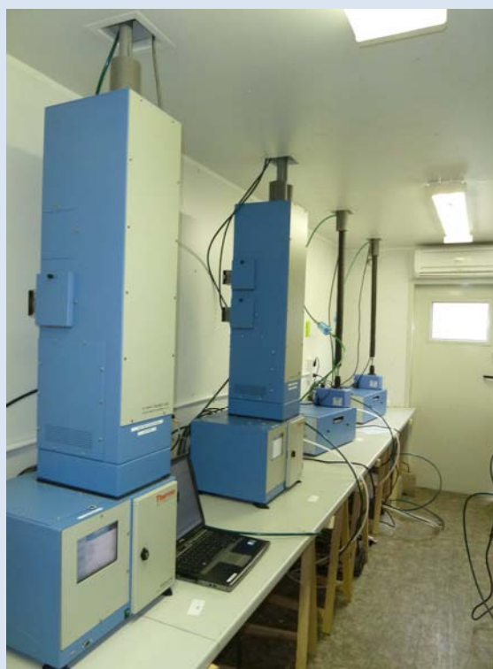
Figure 3: Measuring device TEOM 1405-F Ambient Particulate Monitor (1 st system from left) in measuring station
