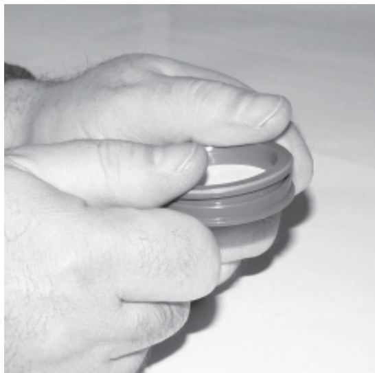
Figure 5-22. Closing the filter cassette.
