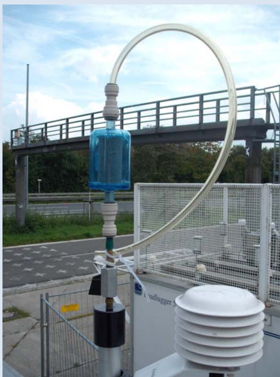
Figure 47: Zero-filter during field test
