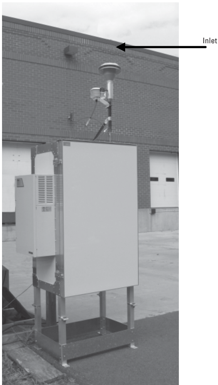
Figure 2-30. Outdoor enclosure with inlet installed.
