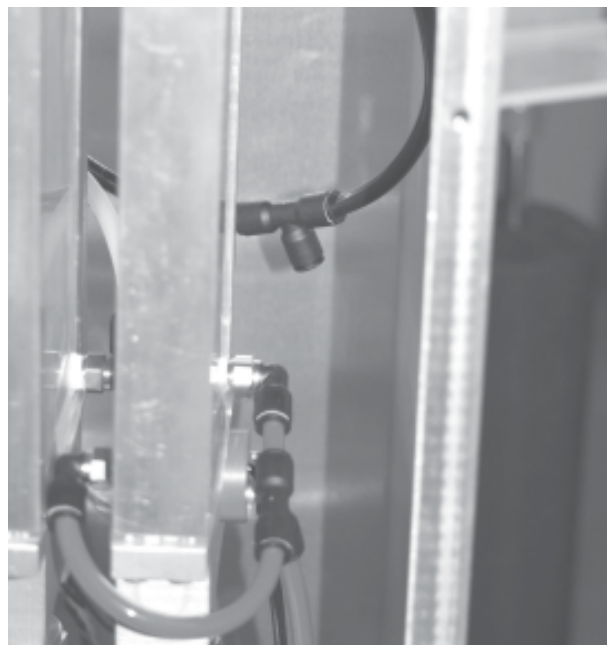
Figure 5-40. Main dryer vacuum line removed from T-fitting.
