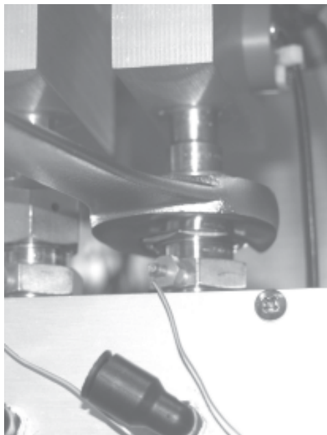
Figure 5-46. Removing a valve Swagelok fitting.
