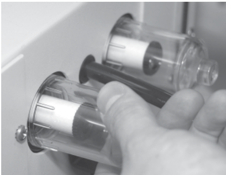
Figure 5-30. Removing the fine and coarse filter covers.
