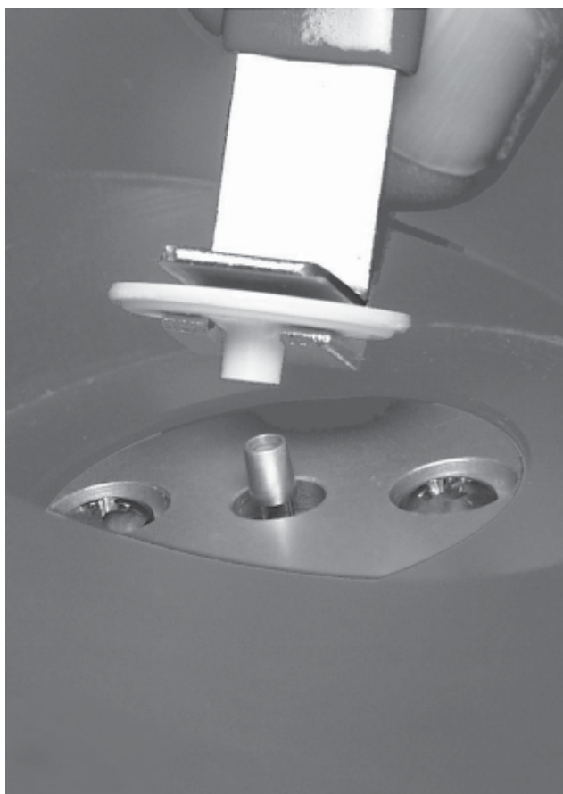
Figure 5-8. Placing the filter on the tapered element.
