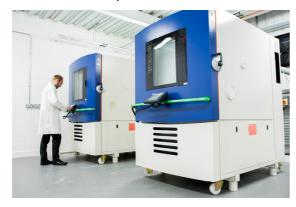
Usually a thermal test is conducted first, to determine the maximum temperature of components and parts under maximum service conditions (i.e. using manufacturer's rating for the device, related to the maximum ambient temperature in service). additional test at 0.9 to 1.1 times rated voltage may also be conducted at this time to determine maximum surface temperature. Again this is related to maximum ambient temperature in service.
